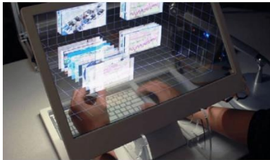
22. Microsoft's see-through 3D display using Samsung OLED screen © Silva 2014 "Glassist ..."
